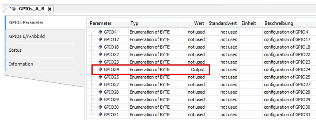
The screenshot shows the 'GPIOs\_A\_B' configuration window in CODESYS. On the left, there is a sidebar with 'GPIOs Parameter', 'GPIOs E/A-Abbild', 'Status', and 'Information'. The main area contains a table with the following columns: Parameter, Typ, Wert, Standardwert, Einheit, and Beschreibung. The row for GPIO24 is highlighted with a red rectangle, showing its 'Wert' as 'Output'.
